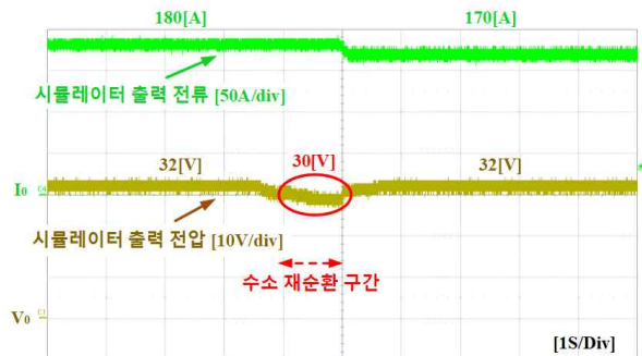
Fig. 28. Output voltage, current waveform of proposed fuel cell simulator
