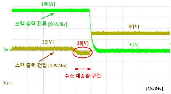
Fig. 27. Output voltage, current waveform of conventional fuel cell stack
